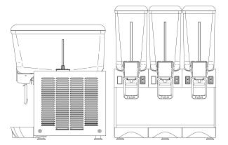
Professional equipment for beverage refrigeration. Available in models with 1 to 3 tanks with capacities of 12 or 20 liters. Fountain pump model (P version).
